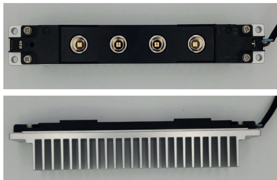
Fot. 2. Modułowy promiennik LED model UVM002A-0401U1-RM o łącznej mocy 9 W (u góry) z radiatorem (na dole), (fot. CIOP-PIB) Photo 2. Modular light-emitting diodes model UVM002A-0401U1-RM with a total power of 9 W (above) with a radiator (underneath), (photo: CIOP-PIB)
